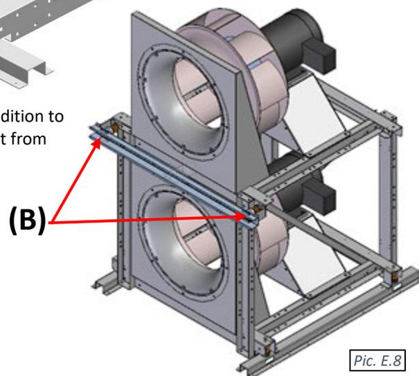
“Split-Deck” dehumidifier (“Double-Decker”) – mechanical field disassembly and assembly
