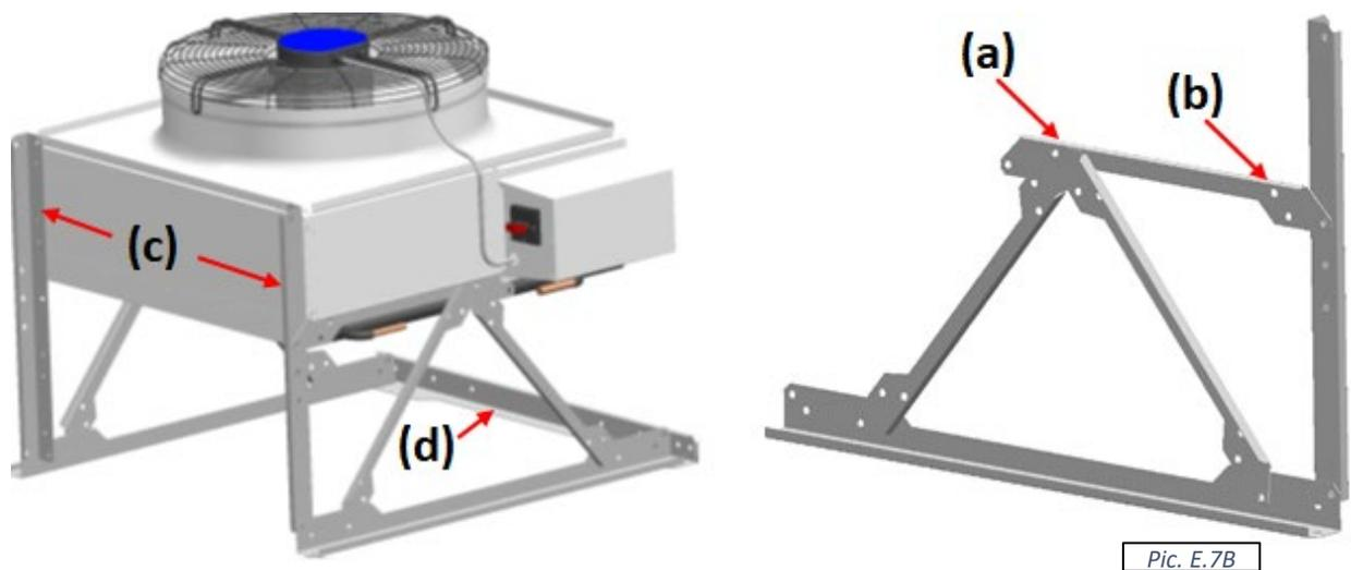
**Horizontal airflow configuration (equipment is mounted on a vertical surface such as a wall.)** In this case, use the same mount kit as above. Note that the mount legs are assembled slightly differently.
